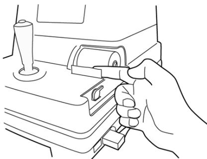
**10** After making sure that the paper comes out, attach the printer cover.
