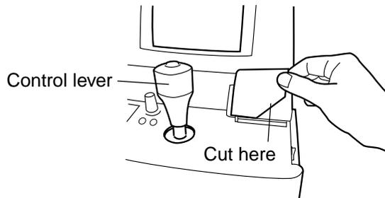
**6** Insert the paper into the printer straight along the paper guide.
